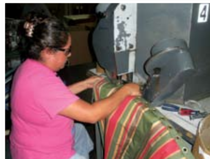
Erika Jimenez applies grommets to edges for hanging a quilted fabric.
